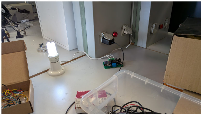
Figura 3.17: Bombilla encendida mediante HomeAssistant.
